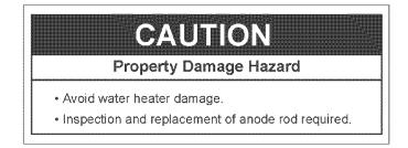
The anode rod is used to protect the tank from corrosion. Most hot water tanks are equipped with an anode rod. The submerged rod deteriorates to protect the tank. Instead of corroding the tank, water ions attack and eat away the anode rod. This does not affect the water's taste or color. The rod must be maintained to keep the tank in operating condition.
